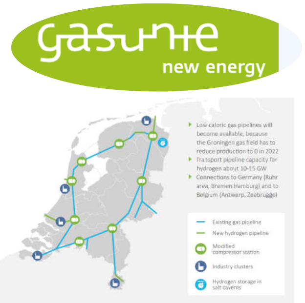
Figure 5 Hydrogen Backbone the Netherlands – Existing natural gas transport pipeline will be converted into a hydrogen transport pipeline that connects hydrogen supply to hydrogen storage and demand in industrial clusters (Gasunie, 2019)
